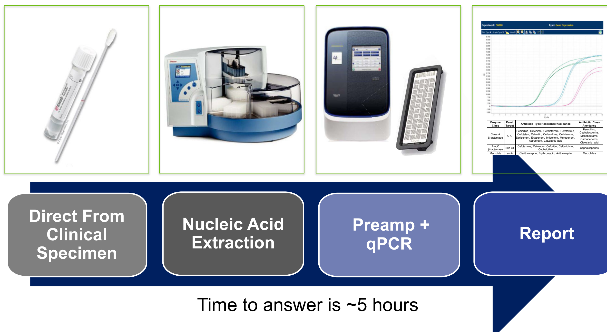
Figure 2. Workflow of the ABRx TM Panel.
